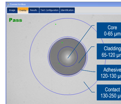
IEC zone sizes for PC polished connectors, multimode fibers
